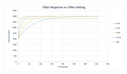
The graph above shows the effect of the filter on response times. Increasing the filter setting increases the measurement output response time.  $T_{90}$  is the time to 90% of reading. The SprintIR<sup>®</sup>-R takes 50 readings per second. The flow rate was set at 0.2l/min.
